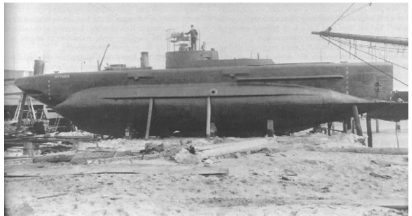
A man stands atop the Defender. Constructed in 1906-1907, this radical design concept was decades ahead of standard submarine development.
